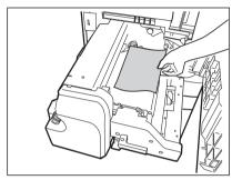
**9** Lift the grip, then turn the knob in the direction of the arrow to remove any misfed paper.
